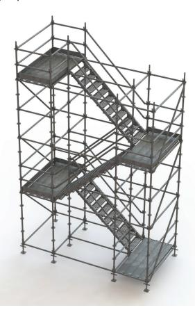
The above figure shows the typical arrangement of the AT-PAC Steel Stair System, which utilizes steel stringer channel with separate tread units which slide and lock into place. Steel Planks form the landings. Bay braces are used for stair handrails and ledgers form the landing guardrails. The Stair tower may be built separately and tied into a scaffold or may form an integral part of the main scaffold structure.
