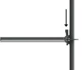
Hammer home wedge to secure in place to create a strong and rigid connection
