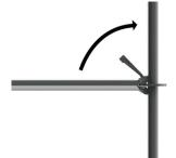
Rotate wedge and insert through hole in rosette
